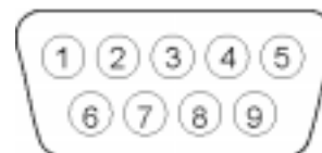
RS-232 Connector Pin Layout.
